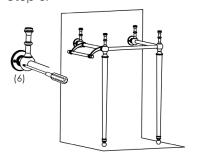
Once assembled, align the console against the wall and secure it with the provided screws (6).
