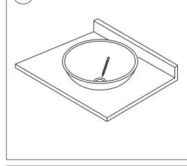
2. Drill a 2.2" (55 mm) hole, or larger if necessary, at the marked location.
