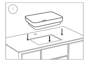
2. Apply a small amount of 100% silicone sealant to the sink's underside rim.
